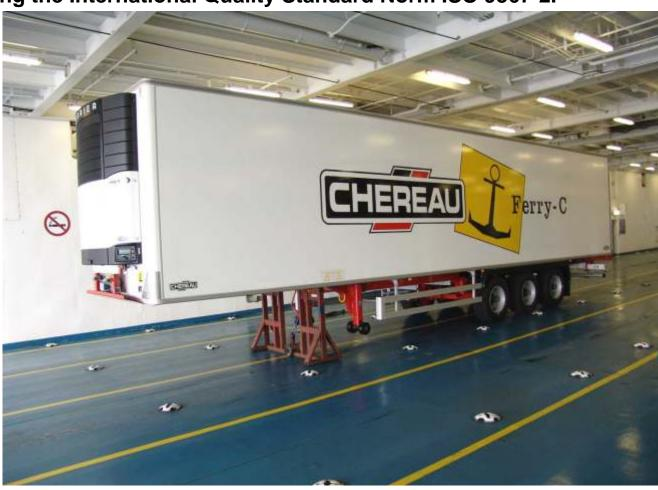
■ Designed for sea transport under bad weather conditions, for which the lashing of the semi-trailer to the deck must ensure the perfect stability of the vehicle and avoiding damage both to the chassis and the bodywork.
