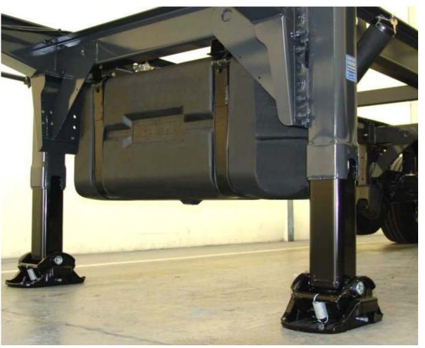
With 250 litres usable capacity, it is the largest capacity refrigerating fluid tank on the market (190 litres for a standard tank), allowing the refrigerating unit to run for 62 hours!
