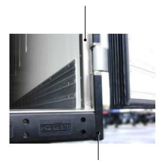
Rubber buffers clipped into the uprights over the full height of the rear frame.
