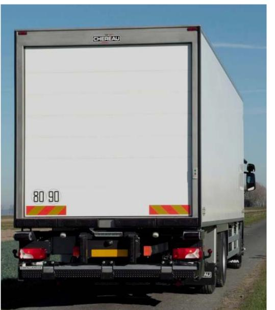
INOGAM bodies are offered with roller shutter type rear closing, with manual or electro-pneumatic opening/closing.
