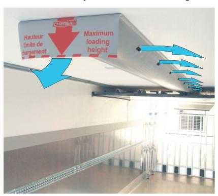
Chéreau has established that the most important thing is not to lower the ambient temperature (which will rise again the instant the doors are open) but to lower that of the body's sides.
