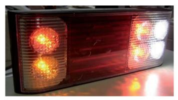
Finally, Chéreau has linked the lights to an intelligent electronic TMU box, which controls the three essential signalling functions (position, stop and direction) and sends information back to the tractor dashboard in the event of a problem.
