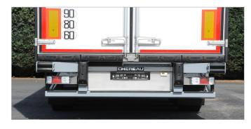
Following a wide range of tests, Chéreau has defined and qualified a new "Full LED" rear light with a high resistance against impacts.
