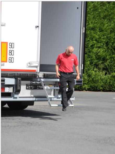
**Static strength up to 250 kg without bending and another 500 kg without breaking.**
