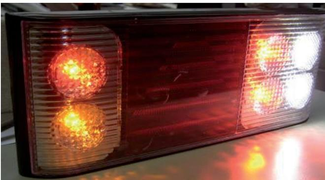
Finally, Chéreau has linked the lights to an intelligent electronic TMU box, which controls the three essential signalling functions (position, stop and direction) and sends information back to the tractor dashboard in the event of a problem.
