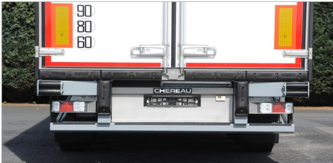
Following a wide range of tests, Chéreau has defined and qualified a new "Full LED" rear light with a high resistance against impacts. The "Full LED" light includes the six main signalling functions: **position, direction, stop, reversing, fog, reflector triangle.**
