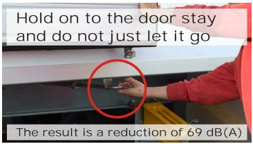
When closing a door: Position the door with the handle open at 90° and take care not to slam it against the bolt..
